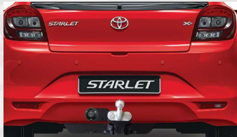
Towbar including wire harness (Not compatible with the rear spoiler)
