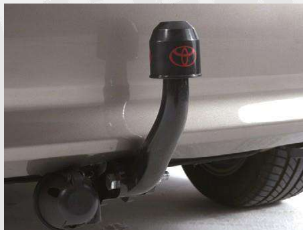
Towing Bar - Fixed (Includes Wiring Harness) Part Number : PZN52A3001 Available : All
